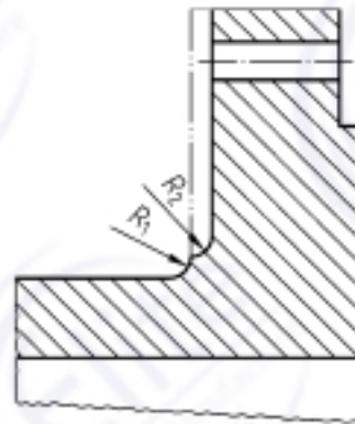
Figure 17 — Minimum hub radius after back facing
