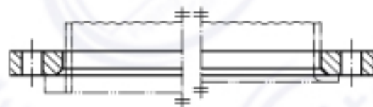
Type 02 Loose plate flange with weld-on collar (see type 32) or lapped pipe end (see type 33)
